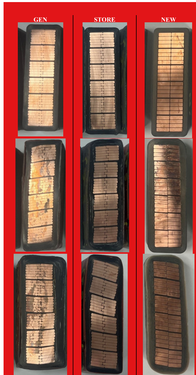
Fig. 2. Dissections of the three coil groups, Top – straight leg portion, Middle – Stress grading region (around the first bend), Bottom – beyond stress grading region.
